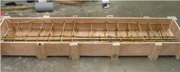
Image 14: Bamboo reinforced concrete beam
