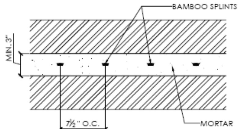
*Image 15: Bamboo reinforcement for cavity wall construction*
